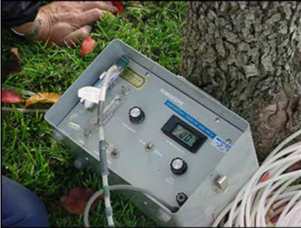
Fumiscope for monitoring fumigant gas in structure.
