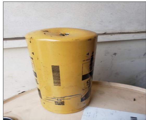
Example of punctured spin-on canister type oil filter to ensure oil is completely drained.
