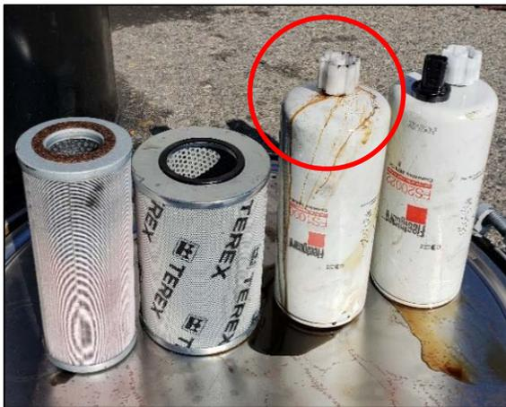
Examples of recyclable metal filters, but the plastic water drain must be removed.
