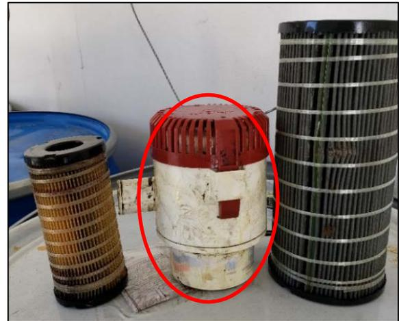
The fuel pump in the middle cannot be placed with recyclable metal or waste filters.
