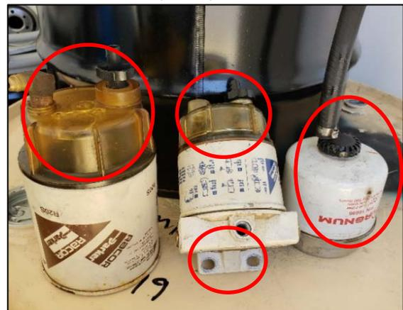
Remove all objects from the filter before recycling (e.g., hoses, housings, fittings, and water separators).
